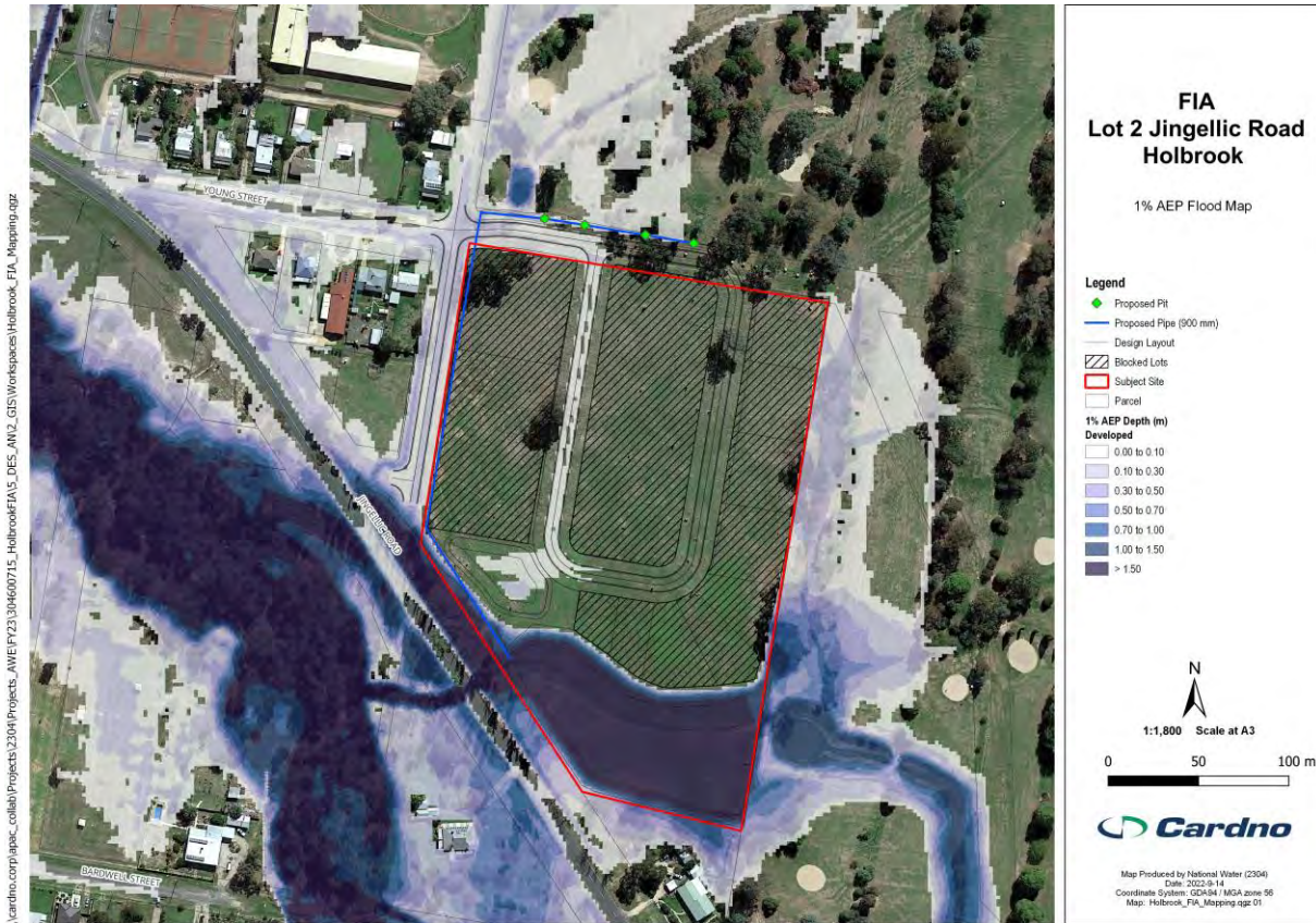
Figure 3-2 1% AEP Flood Depth – Developed Conditions
