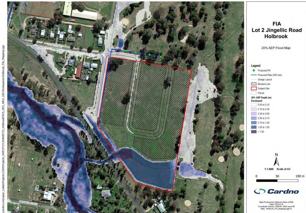
Figure 3-4 20% AEP Flood Depth – Developed Conditions
