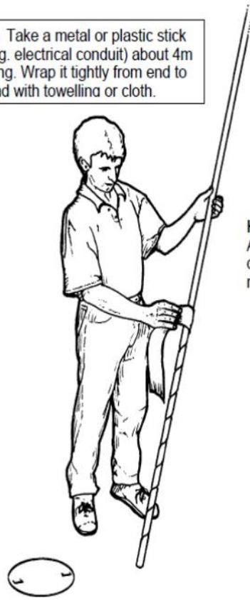
2) Wearing rubber gloves, remove the inspection cover (inlet end) and insert dip stick all the way to the bottom of the tank.
