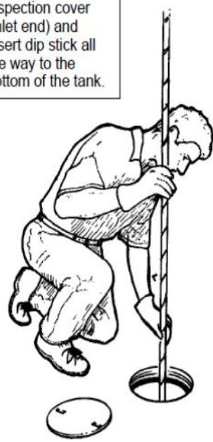
3) Withdraw it completely, observe the size and position of the scum mark (bottom) and the sludge mark (top).
