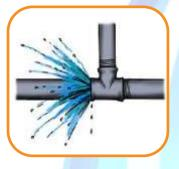
If you have a leaky or burst pipe or a dripping tap you will need to turn off the water supply at the meter before repairs are undertaken.
