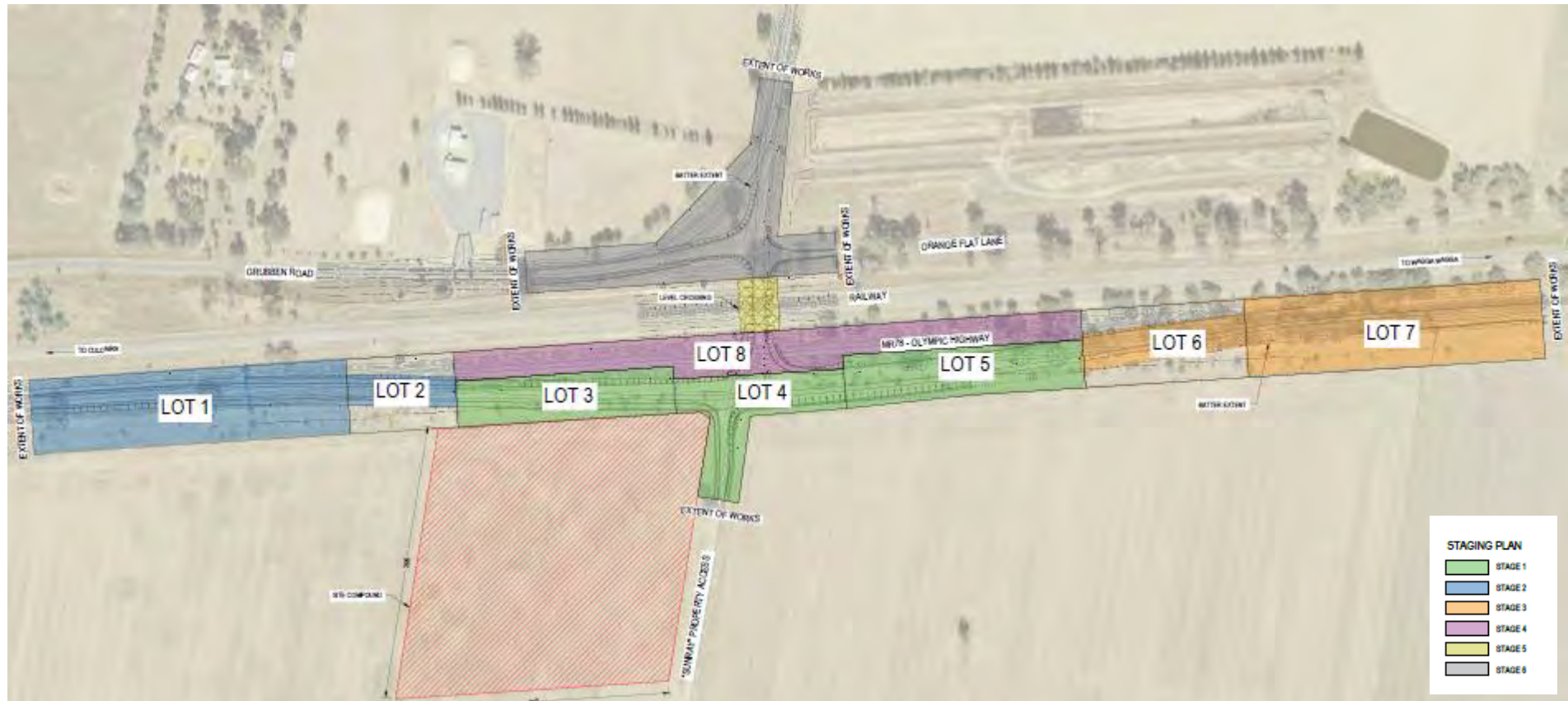
Figure 1 Lot production to construct diversion to enable culvert construction
