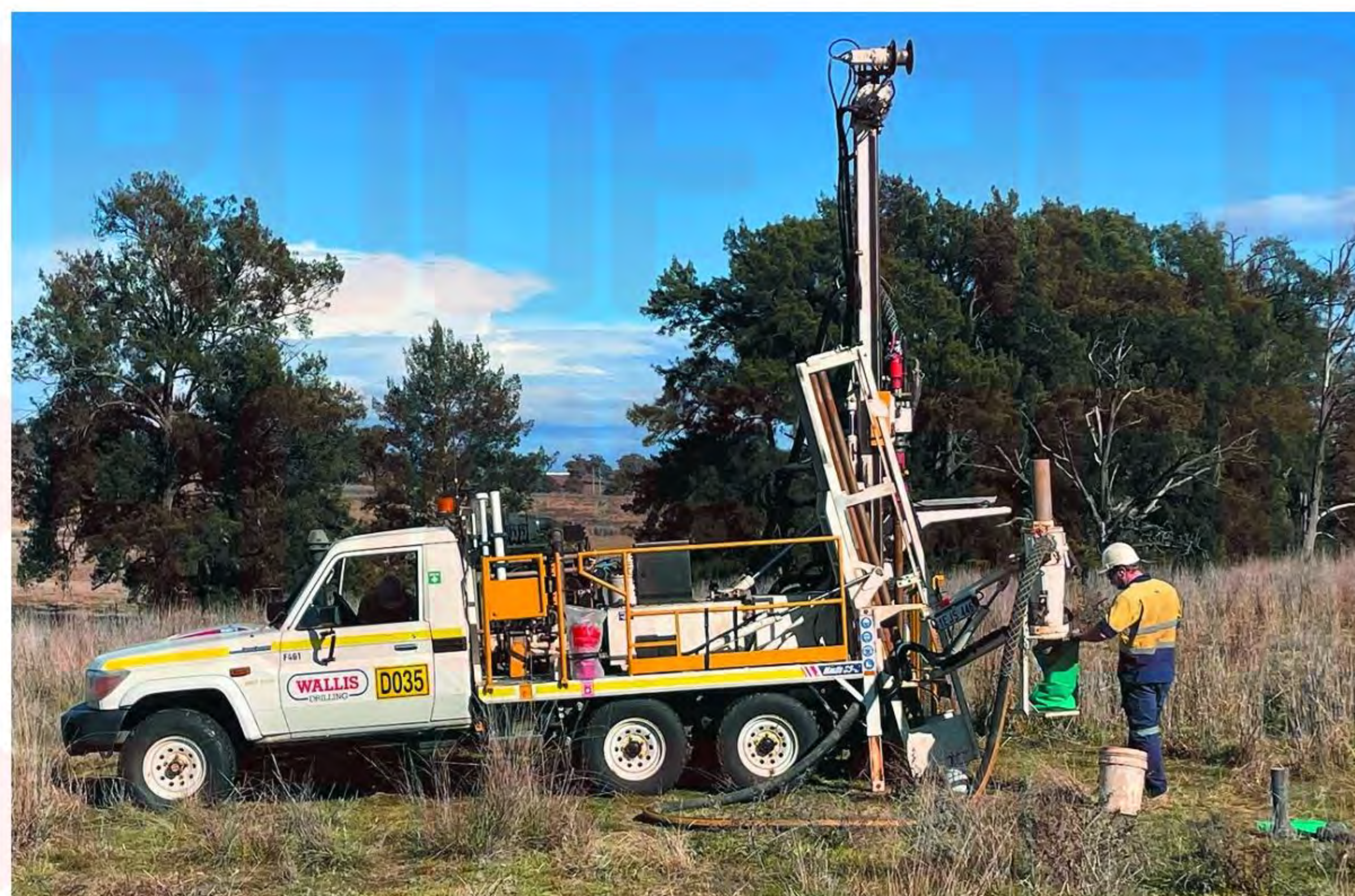
FIGURE 2: typical air-core drill rig that will be used for the proposed program.
