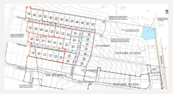
Figure 4 - Proposed subdivision layout plan - Stage 3.1 & Stage 3.2
